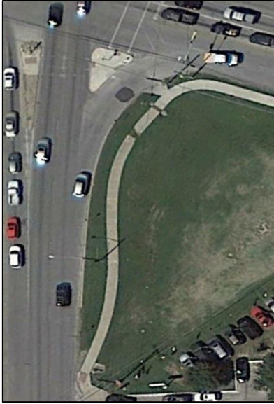
Figure 3. Example of shared lane with island
