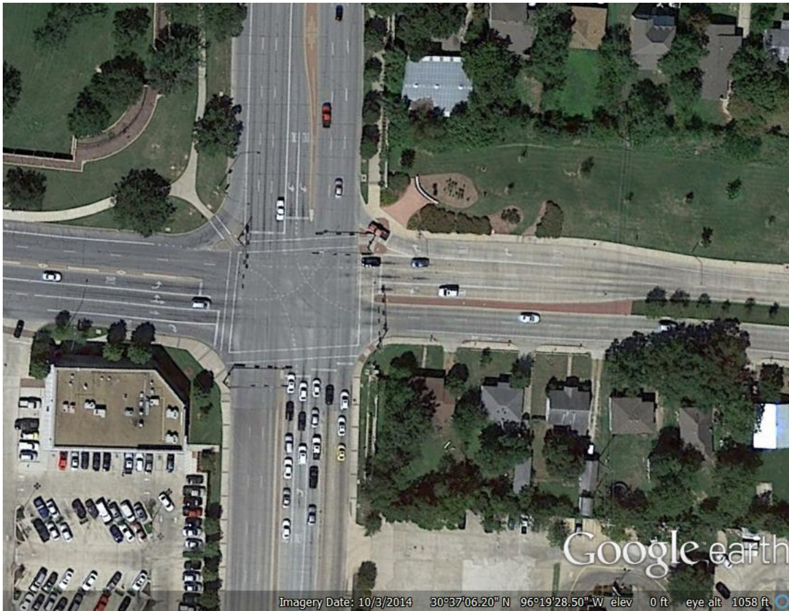
Figure 7. Example of exclusive right-turn lane (eastbound approach), shared lane (northbound approach), and right-turn lane with island (westbound and southbound approaches)—note southbound approach crosses a bike lane after turning to west), assuming north is to the top of the photo.
